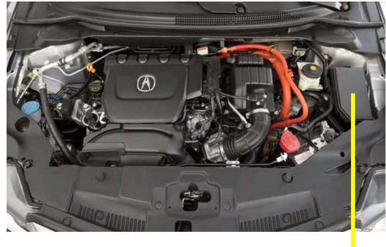
Underhood Fuse Box
